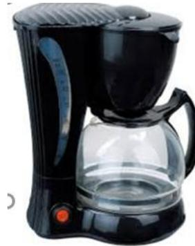
A single-time use paper filter is put into the percolator of the coffee machine and the ground coffee placed in the filter. Cold water is filled into the coffee maker. Once the machine is switched on, the water is pumped to a heating coil. The heated water runs through a small pipe on top of the percolator and drips onto the coffee in the filter paper. The coffee passes through the percolator and drips into the coffee pot beneath. After about 5 minutes, the process is complete.
